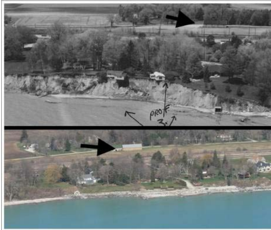
Figure 21. The Lake Michigan shoreline in Racine County in 1976 (upper) and 2007 (lower). Large black arrows point to the same barn in each photo. In 1976 water level was high and severe erosion was taking place. By 2007 all the shoreline here had been armored with rip rap or concrete. (Source: D. Mickelson).
