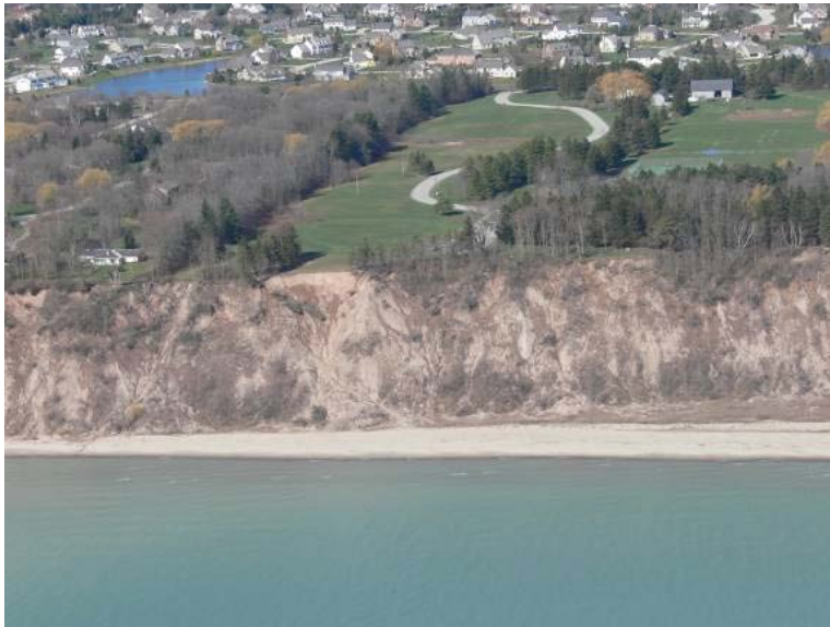
Figure 3. Aerial photo of the Lake Michigan shoreline in southern Ozaukee County showing a high, eroding bluff. Virmond County Park is in the northern part of the photo (Source: D. Mickelson).
